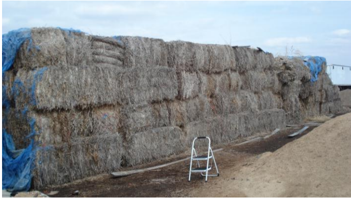
(a) Bale stack in Griggsville, IL. Bales were covered with a tarp for 12 months and ripped tarp for the next 12 months.
